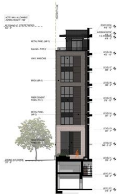
COURTYARD ELEVATION (SOUTH)
