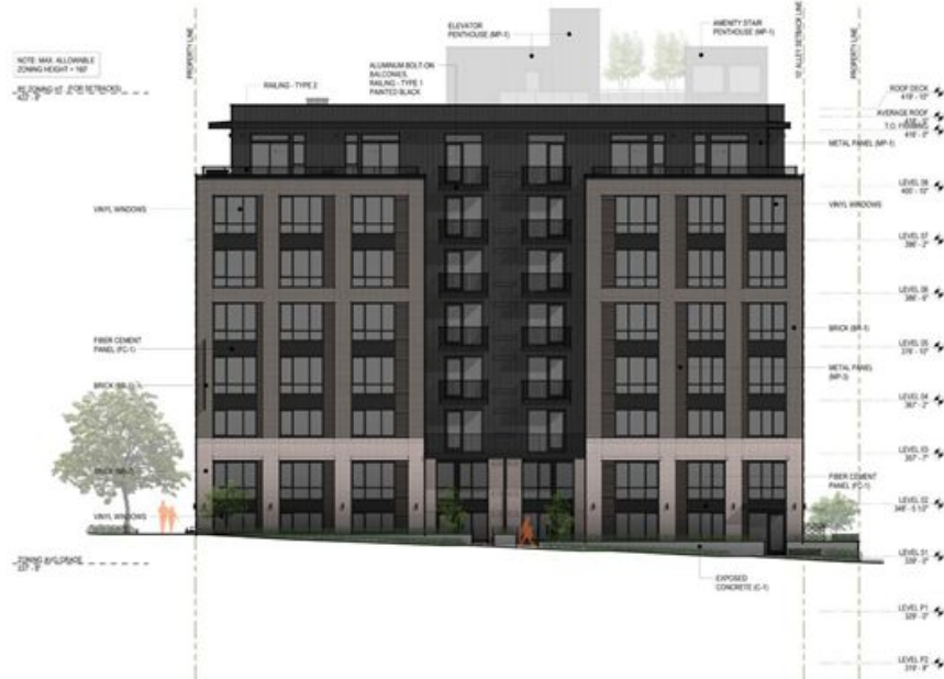
SPRING STREET ELEVATION (SOUTH)
